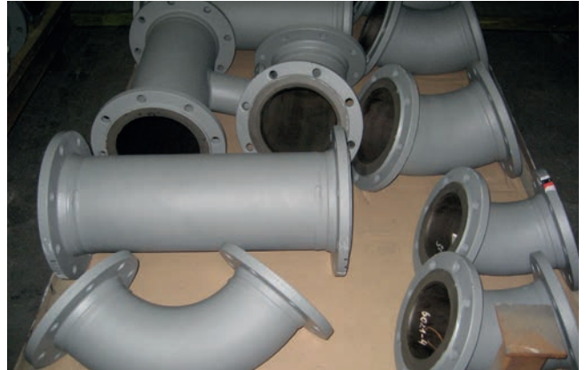
Rubber lined small parts of a pipe
